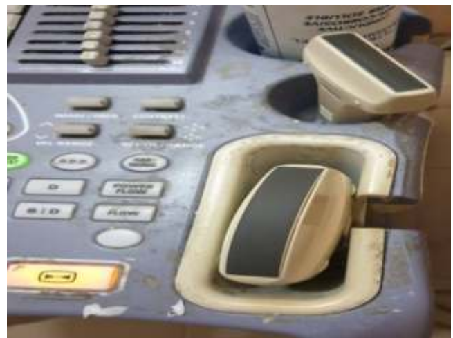
Figure 1: Caked gel stains on control panel
